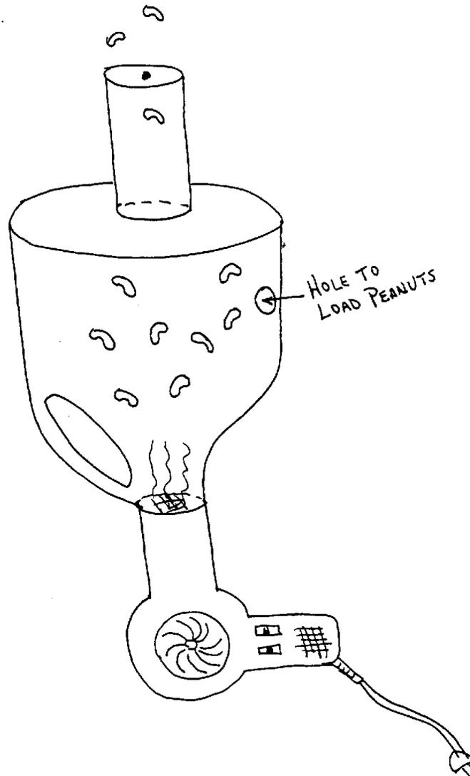
Directions for making the Holy Spirit Power Shooter: Cut a hole in the bottom of a milk jug. Make the hole large enough for a cardboard tube from paper towels or bathroom tissue to fit snugly into. At the mouth of the jug, cut a hole large enough so the nozzle of a hair dryer fits securely. Seal the dryer nozzle to the jug with tape. Cut a small hole in the side of the jug where the packing peanut from Gordy's nose can be dropped in.
